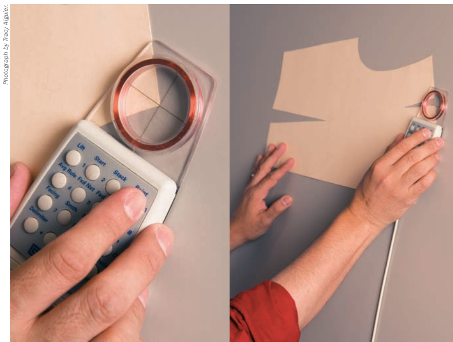
Digitizing a pattern using a Gerber digitizer
